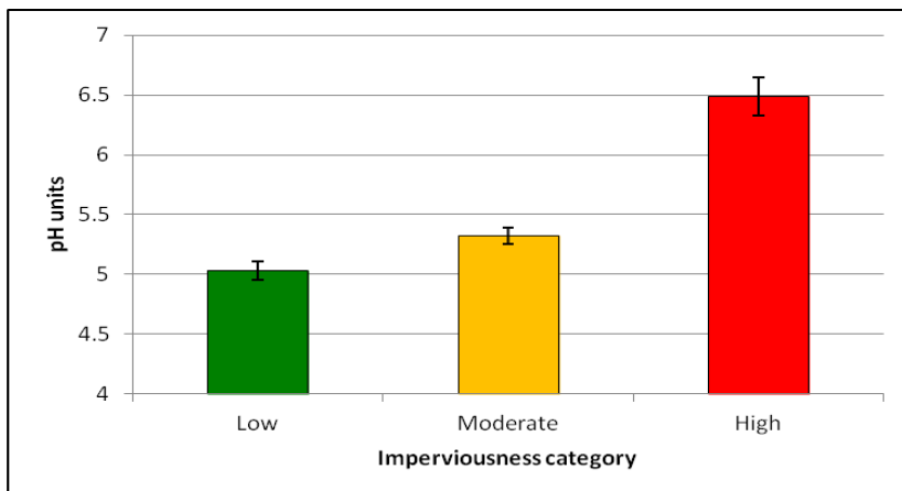
Figure 3. Mean ( \pm SE) pH of composite soil samples collected from low, moderate and high impervious sites in the Georges River catchment (low n=18, moderate n = 17, high n=24)
